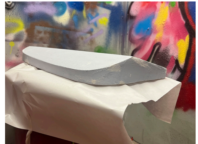
CNCing both the the interior and exterior shapes in EPS foam and using a foam coating on the exterior for durability.
