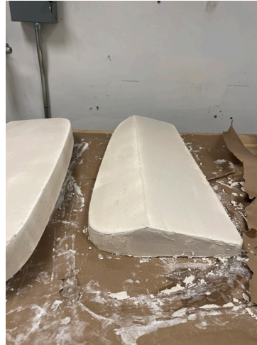
CNCing both the the interior and exterior shapes in EPS foam and using a foam coating on the exterior for durability.
