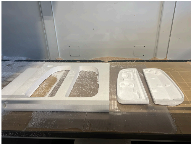
CNCing both the the interior and exterior shapes in EPS foam and using a foam coating on the exterior for durability.
